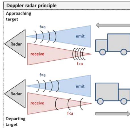
Fig. 4: Doppler radar measurement principle based on the Doppler Effect where  $f$  denotes the radar frequency.
