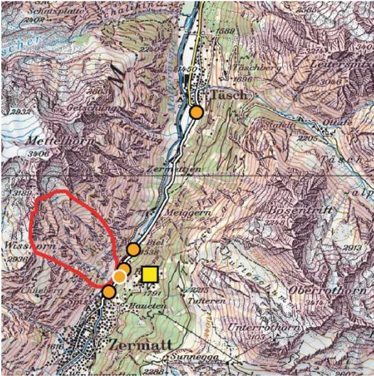
Fig. 1: Location of Zermatt, Täsch and the monitored avalanche gullies (red outline). Areas shaded in pink are steeper than 30 degrees. Orange dots are stoplights with cameras (white outline = no camera), the radar system is placed at the yellow square. Map source: Swisstopo
