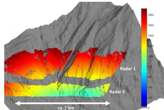
Fig. 2: Simulated radar coverage of the Zermatt avalanche detection system. Areas seen by the radars appear in color. Colors indicate distance to the radar, dark red is approximately 2,000 m.
