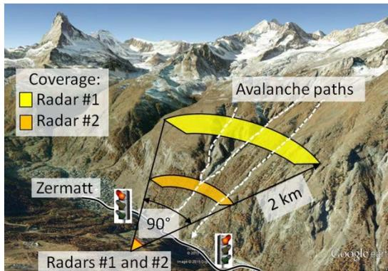
Fig. 3: Avalanche detection and alarm system overview, Zermatt
