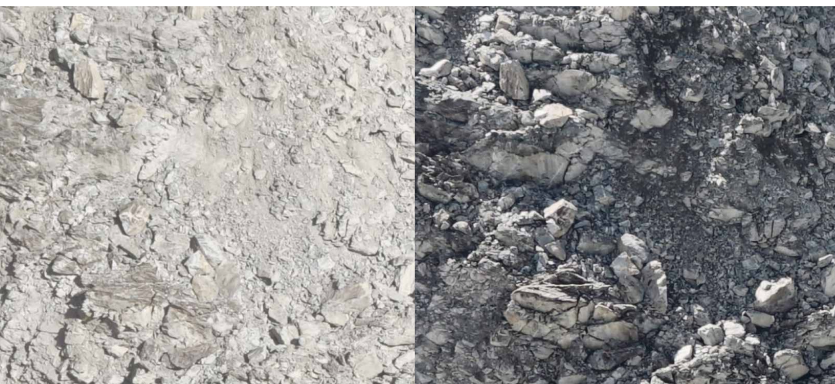
Figure 4: The same image section left (8 AM) and right (12 PM) with different light and shadow conditions. The automatic evaluation algorithms can independently distinguish between displacement and changes in light.
