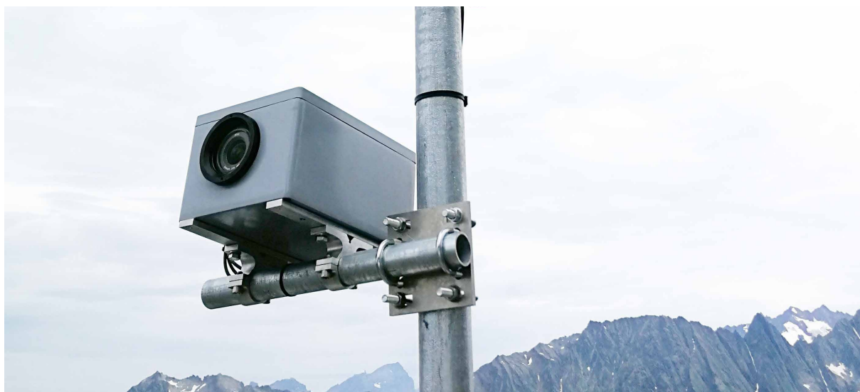
Figure 8: Deformation camera station at Randa installed to monitor Bis glacier from the valley bottom.
