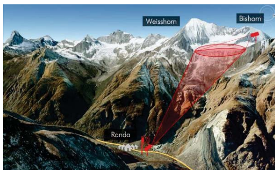
Figure 1: The municipality of Randa in the Matter valley at the base of Weissshorn and Bishorn. The doppler radar and one of the high-resolution cameras are mounted on the opposite side of the valley. The second camera is installed above the icefall, providing a good view of the sérac zone from an elevated position.
