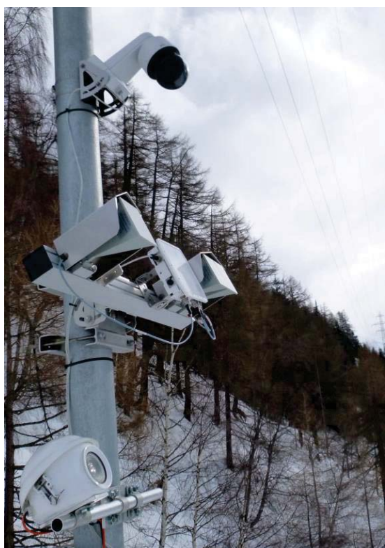
Figure 2: Radar systems (middle) and high-resolution camera looking up at Bis glacier near the municipality of Randa.
