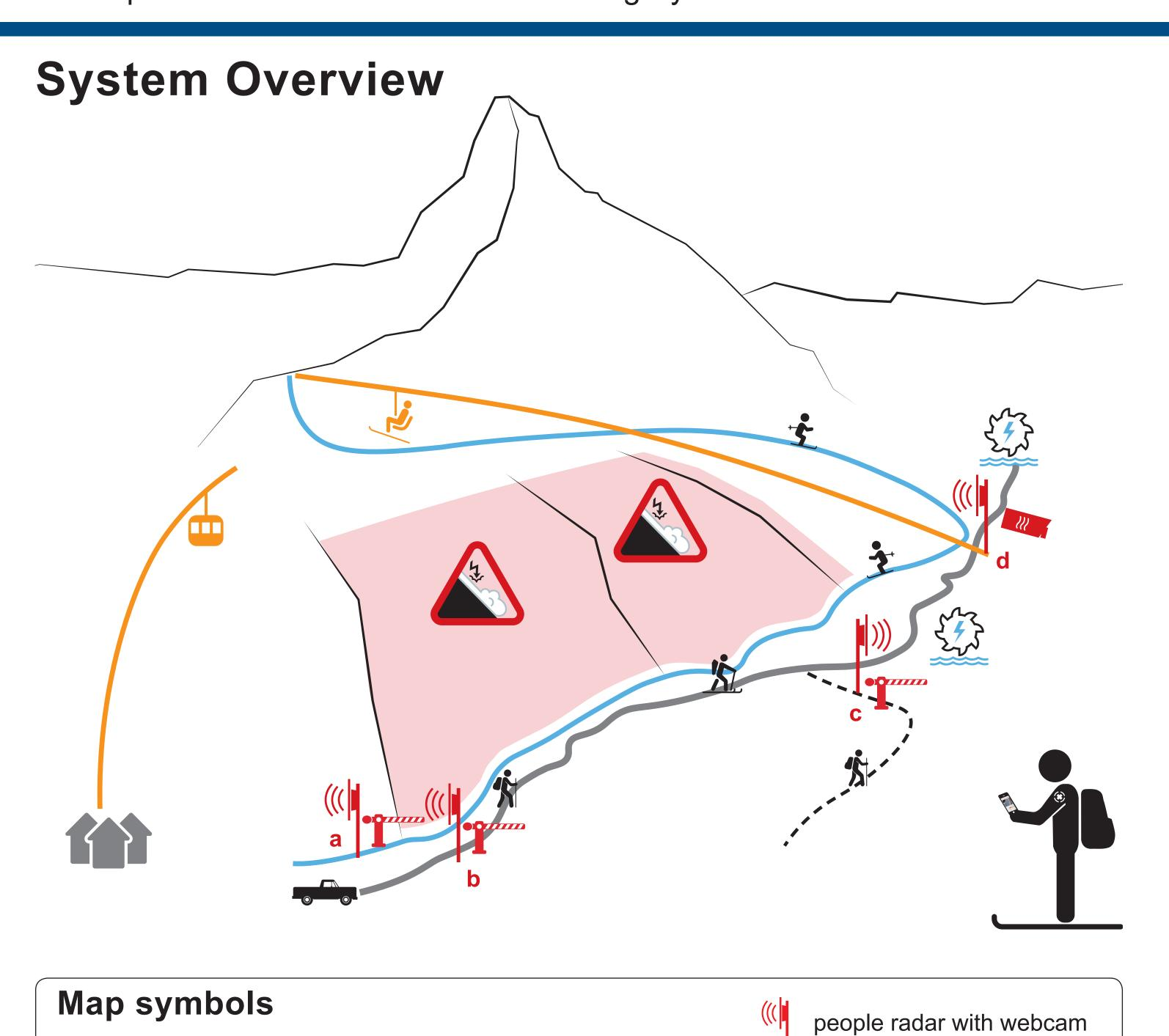
We designed a modular system based on detection stations, cloud servers for data processing and an online data portal. Each detection station includes a people radar, camera, data logger and communication device. The radar triggers the camera at detection, which automatically takes a picture (or a series of pictures). Cameras can also be used for live views any time.
