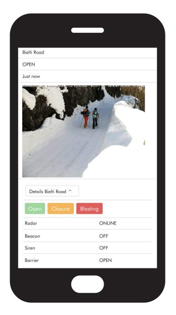
with control System smart phone (left) to close barriers ("Closure" state) and activate sirens and beacons ("Blasting" state). Blasting triggers a local alarm if a person is detected despite closed gates. Online map tracker with associated pictures event and characteristics.
