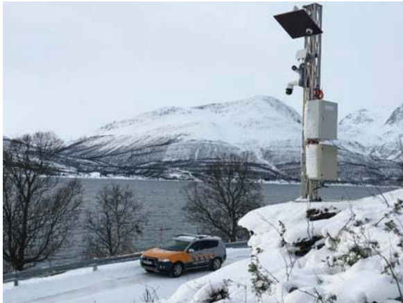
Figure 3: Radar installation (February 2017). To verify detections, a remotely controllable PTZ camera and a thermal camera were installed additionally. Photo: Andreas Persson
