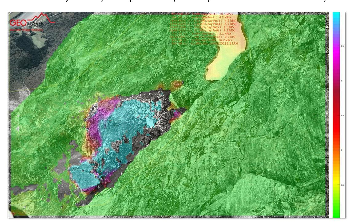
indicated significant displacements. In the following weeks, the unstable area increased in size with simultaneously accelerating displacement rates until the slope failed on September 5, 2019.
