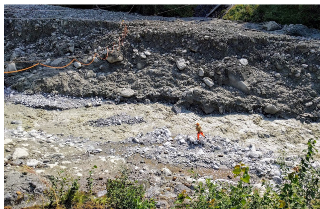
Figure 3: Gauge radar station (station A) across the Bondasca river with several meters debris flow deposits in August/September, 2017.
