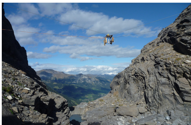
Figure 2: The gauge radar monitors the discharge of the glacier plateau at Trüebach river; a tributary to the Simme, flowing to the valley village Lenk.
