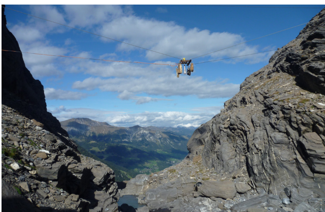
Figure 2: The gauge radar monitors the discharge of the glacier plateau at Trüebbach river; a tributary to the Simme, flowing to the valley village Lenk.
