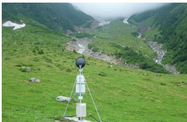
Figure 2: Radar measurements are used to detect movements in the rupture zone of the debris flow.
