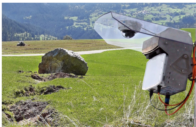
Figure 2: The rockfall radar detects falling rocks and automatically activates a webcam which takes pictures of the event.
