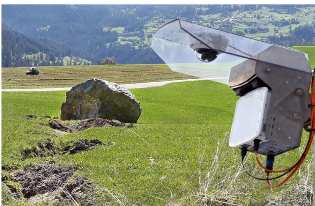
Figure 2: The rockfall radar detects falling rocks and automatically activates a webcam which takes pictures of the event.
