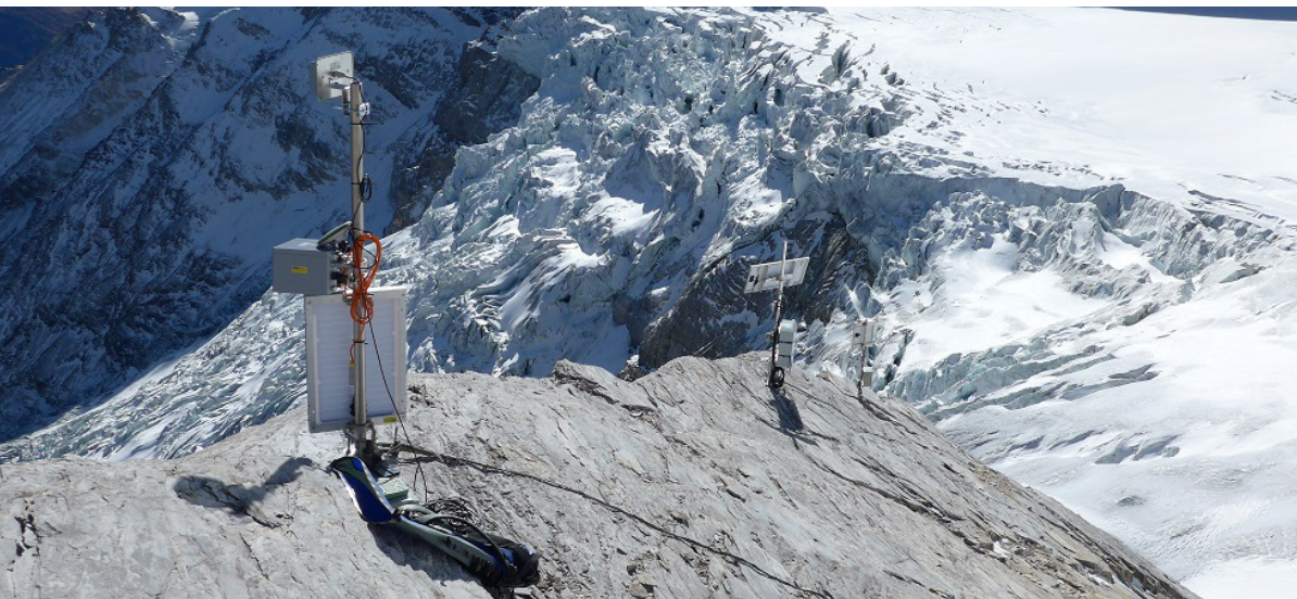
Title Page: A high-resolution camera is installed at the valley bottom and observes the steep part of the Bis glacier.
