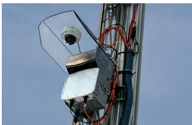
Figure 2: The avalanche radar reliably detects avalanches in any weather and at any time of day and triggers camera images.
