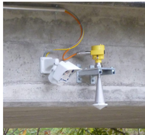
Gauge radar and event camera Steinach (above), Gauge radar Bondo (below), both Switzerland
