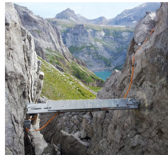
Crack meters Limmern (above), crack meters with slope failure Tafers (below), both Switzerland
