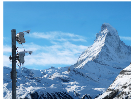
Double Avalanche radar setup Zermatt, Switzerland (above), Avalanche radar at Loveland Pass, Colorado, USA (below)
