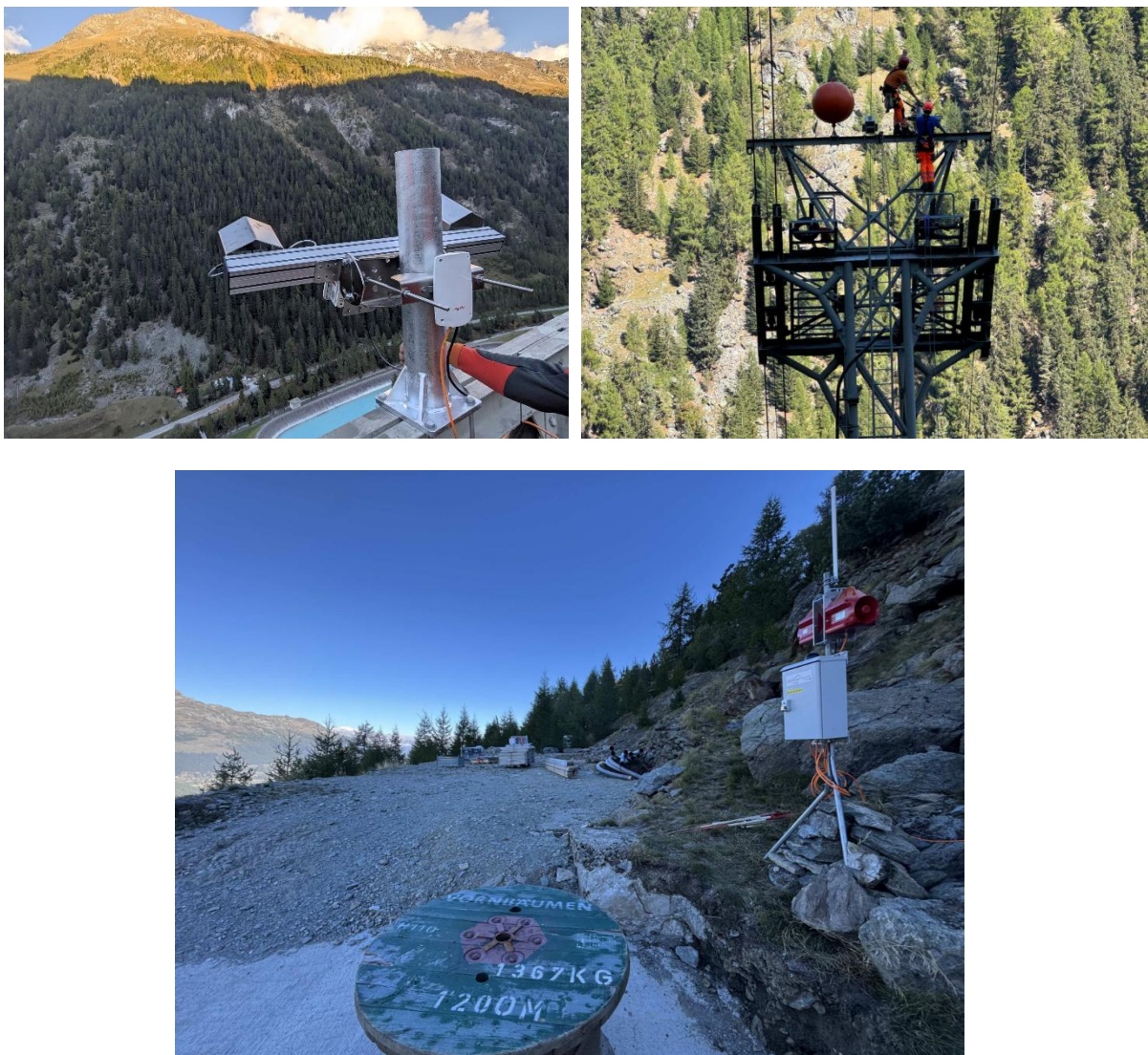
Figure 2 Aspects of the radar monitoring location showing hardware, tower to which the radar was mounted, and the mobile alarm system
